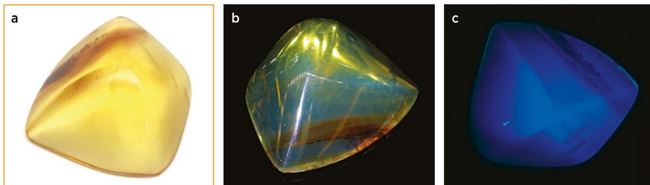
**Figure 5:** This light yellow Burmese amber (a) appears greenish in daylight-equivalent lighting (b) due to its blue long-wave UV fluorescence (c). The sample weighs 20.21 ct; photos by X. Jiang.
